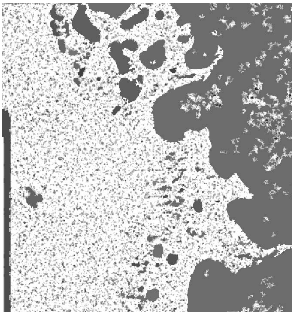
Fig. 9. Image quality, the brighter the points the better the quality. Connected unusable points have the same color.
